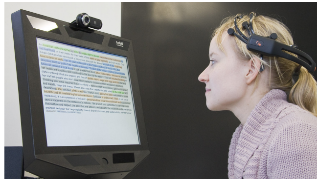
Figure 1. The experimental setup. The user sits in front of an eye tracking device while reading text. A web cam or neuroheadset track displayed emotions which are then annotated in the text.
