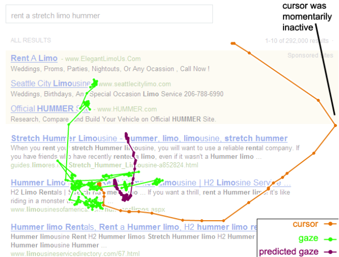
Figure 6. The cursor position (orange), the gaze position predicted by the linear regression model (purple), and the gaze position as determined by the eye-tracker (green) are drawn over the SERP presented to the subject following the query “rent a stretch limo hummer” from our study. The figure omits the right and left columns of the SERP.
